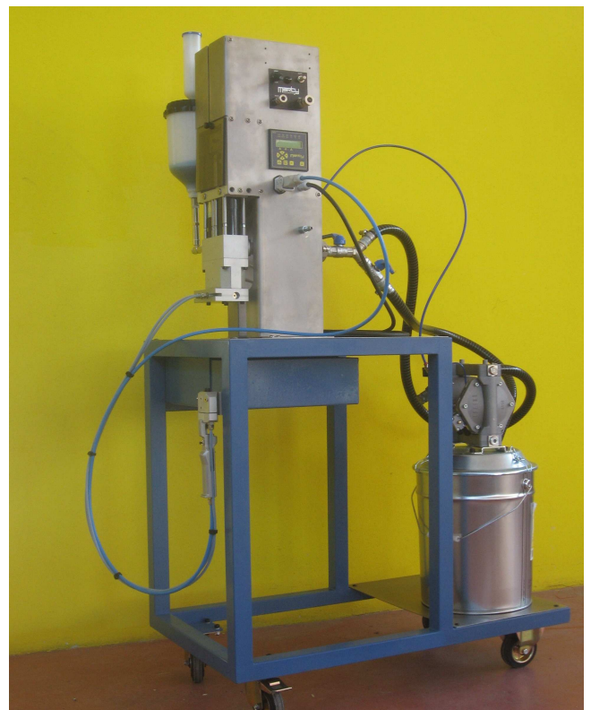
Dosage plant paired with membrane pump for resin and Lt. 2 tank for hardener.
