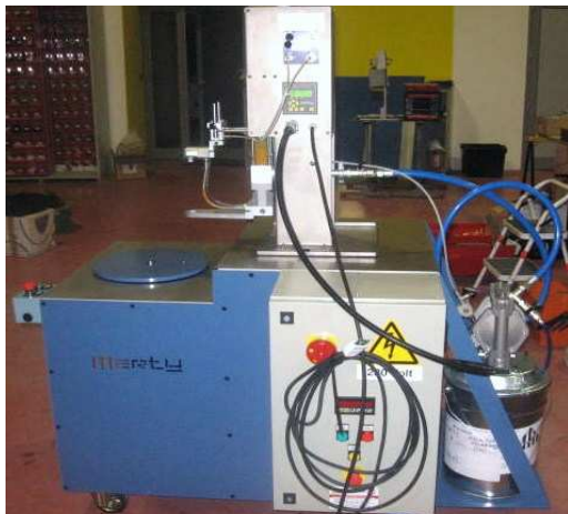
Dosage plant paired with membrane pump and rotating table.
